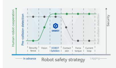
\*Measured results: DOBOT SafeSkin can avoid collision when the robot moves at a low to medium speed; it can reduce collision damage by 90% when the robot moves at a high pace, so it conforms to the safety standard of a collaborative robots.
